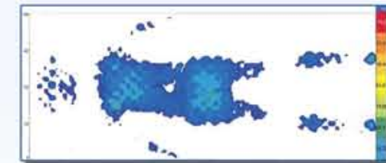
Without Breeze Male, 68 years old, 6'0 tall, 190 lbs., Back lie flat Average pressure = 18.02 Peak pressure = 43.4
